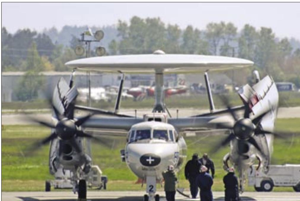
*The E-2C Hawkeye is the US Navy’s all weather, carrier based tactical airborne warning and control system platform.*
