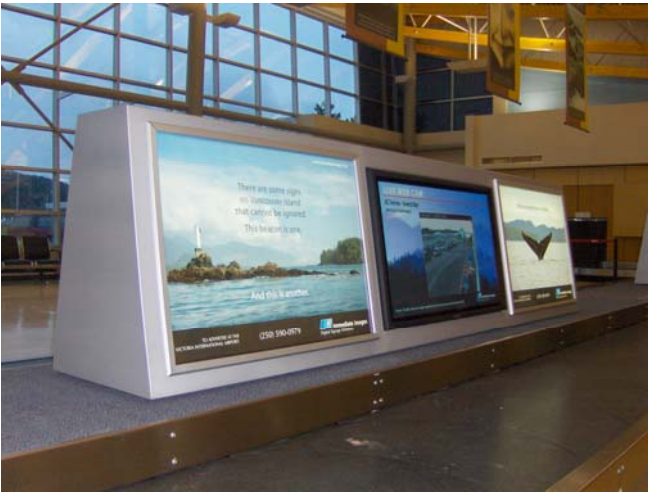
South Carousel A-Frame – two backlit panels on either side of a 50” plasma display.
