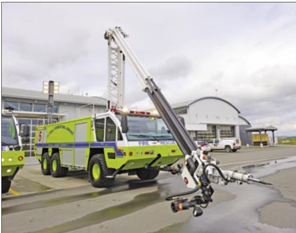
The new Rosenbauer fire truck is capable of piercing the wall of an aircraft to inject fire retardant foam.
